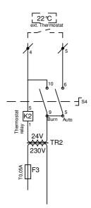
Internal circuit: Inside the heater there is a 24V transformer and a relay. The transformer supplies the 24V signal for the thermostat circuit and the relay gives the electronics the heat demand. This relay is also a boundary for external signals that can damage the electronics.
