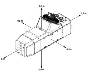
(possibility of) materials within 5m from the front of the heater. See the drawing for the safe distances.
