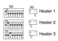
Change the settings from the switches on the control unit in the heater.
