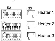
Each heater needs his own unique number to recognise the heater by the room thermostat. The number of the heater can be set by the micro switch on the heater control HC in the heater. The number at the upper position of the switch is the given number for that heater. Make sure that each heater has is own unique number. If more than one heater have the same number the system does not work.
