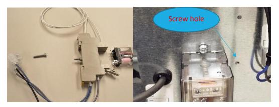
Figure 2: Remove relay from relay support.
