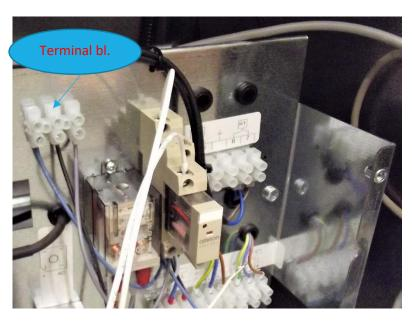
Figure 4: Relay+ terminal block directly on the appliance
