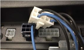
Insert the brown and blue wire into the middle 2 holes of connector J3 until they snap in.
