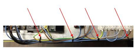
Insert the connector again and attach ty-wraps to fix the new cable.
